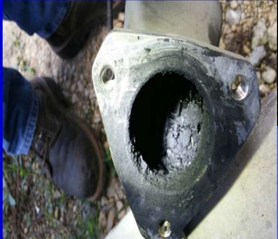
EGR Cooler with Carbon Build Up
